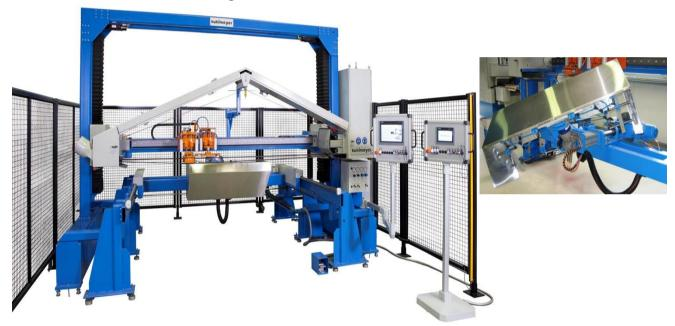
By using the fully automated solution "Robotec" the production time can be reduced with a factor of 2,5. Even with the overlapping of preassembly and setup on other workpieces by the operator, the total output on finished parts can be raised up to a factor of 3, compared with a manual production. At least, the quality is close to 100% due to a maximum repeatability in grinding by programmable steps and procedures.
